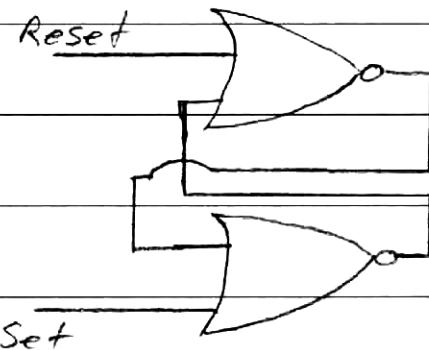
The device shown is a simple RS-NOR flip-flop, its data can be reset by a signal to the Reset control line and a new value supplied through the Set control line.
