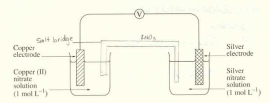
(a) Complete the above diagram by drawing a salt bridge.
