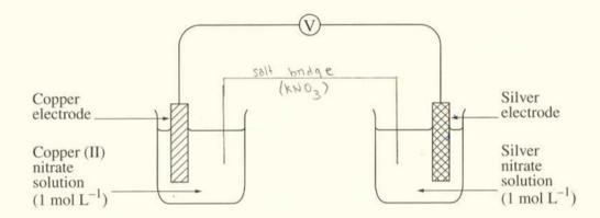
(a) Complete the above diagram by drawing a salt bridge.
